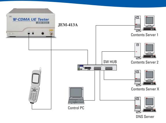
JEM-413A switches a bearer for AMR, packet, or multi-call (option) by conducting simple operations from the terminal without changing the scenario so that terminal application software developers can perform tests under conditions similar to an actual-base station.
